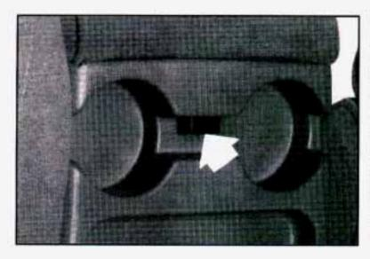
To raise or lower the center console, press the button between the beverage holders.
